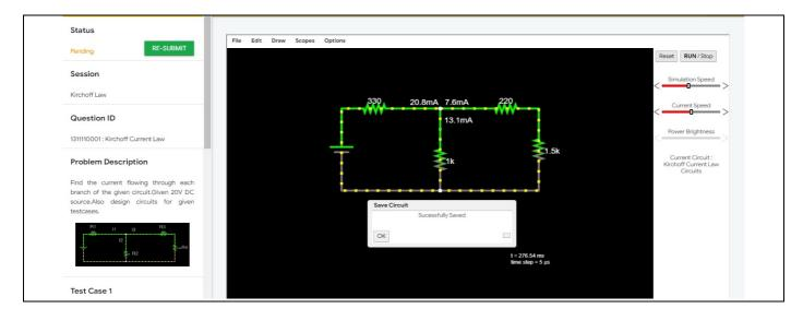
Learner can also design different circuits for the given test cases in the same work space and label them with text boxes.
