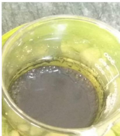
Fig. 2. Mixture at Ice-bath at below 2°C for about 1 hour
