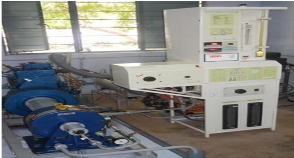
Figure 1: Single Cylinder Multi-fuel variable Compression ratio computerized IC Engine Research test setup
